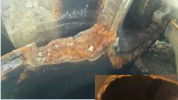
Corrosion Caused By Improper Gasket Cutting
