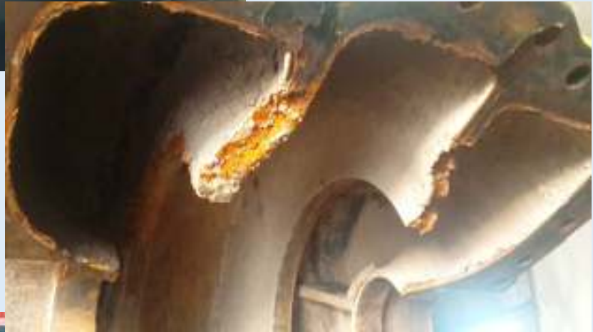
Corrosion Caused By Improper Gasket Cutting
